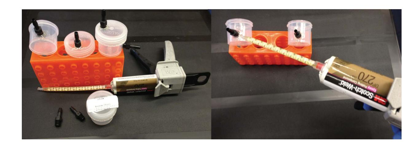
Solder holes for electrode inserts. Insert the smaller end into bottle while plastic is melted. Epoxy only the outside squares of fittings to bottle, making sure to leave the fitting interior clear for electrode insertion. Allow to dry overnight.
