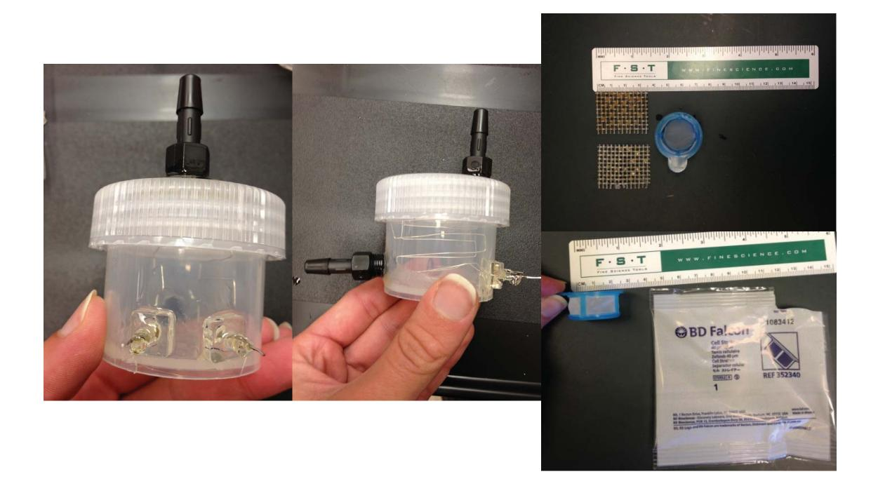
If you are clearing samples with fluorophores, lightproof your chamber prior to use with aluminum foil 'tape'. Place sample in BD "cell strainer" between two mesh squares prior to running ETC setup
