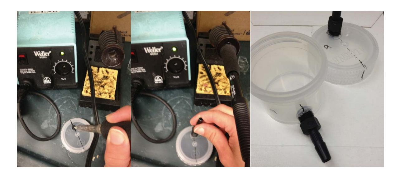
Apply epoxy to the junctures (inside and outside bottle) of the barbed wire fittings. Avoid getting epoxy into the inlet and outlet. Let dry overnight with each epoxy application.
