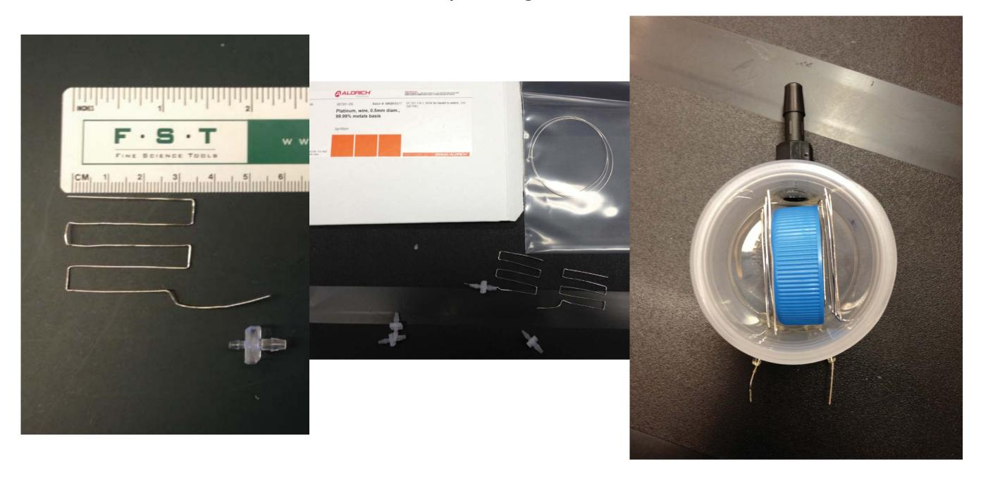
If you are not dealing with samples containing fluorophores, your chamber is ready for use as is... Place your sample into a BD falcon "cell strainer" flanked with mesh between electrodes prior to running in ETC setup
