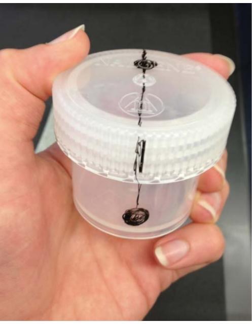
Solder holes into Nalgene bottle and screw in barbed fitting while plastic is melted.
