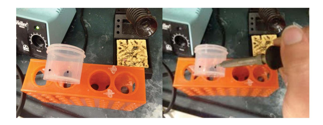
Fabricate electrodes out of .5mm Pt wire and insert into electrode fittings delicately. Ensure that the electrodes are spaced to fit the sample cup snuggly (the same size as a 50mL conical tube top). Fill dead space in electrode fittings with epoxy. Allow to dry overnight.
